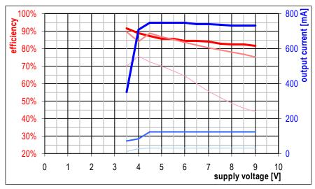
Kennan\_III (AX2002) modified for medium currents: R330, 3k6,  $C_{IN}$  22 $\mu$ ,  $C_{OUT}$  47 $\mu$ , reinforced ground trace, multiple connections to the bottom ring.
