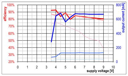
Original Kennan\_III with AX2002 but R330 instead of R220 and connection from FB pin to R330 cut and reconnected via 3k6 allowing analog dimming. At input voltages below about 5V the function was unstable and the LED flickered randomly.
